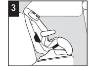
Connect and tighten harness straps prior to installing in vehicle. Place child restraint flush against the back of the vehicle seat forwardfacing in the back seat. The recline position is to be used only to install the child restraint flush against the back of the vehicle seat back, if needed. 35 continued on next page.
